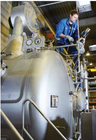
Checking the pressure vessels on a machine with THEN-AIRFLOW technology. It uses an air cushions rather than dye liquor to transport fabrics in the machine, reducing water consumption by 75% and processing times by about 50%.
